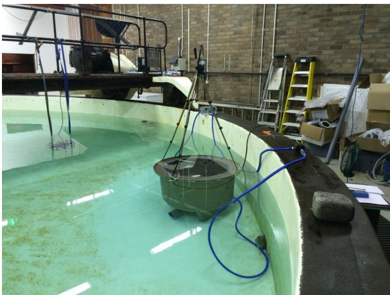
Above: Respirometer positioned in the annular tank 2 meters from the speaker, with the pumping system to circulate water in the chamber in place.
