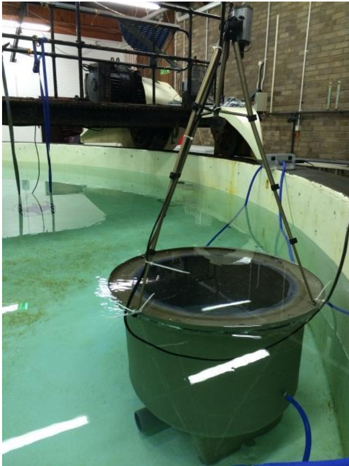
Above: Respirometer in the annular tank with the HD megapixel camera positioned above the chamber to film the fish.
