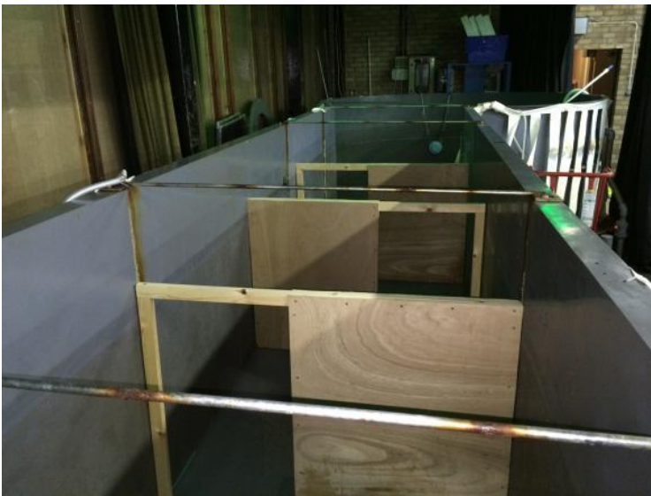
Above: Soundproof baffles installed in the dumbbell tank raceway prior to additional bubble wrap being added.
