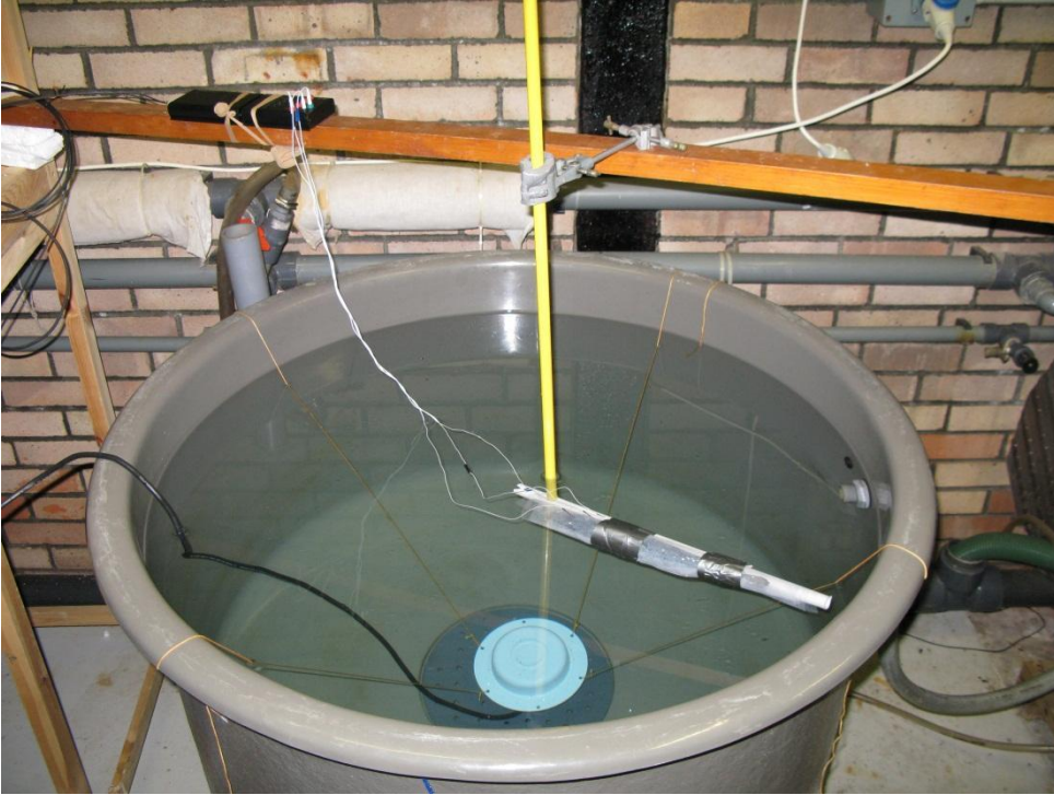
Above: 1 m diameter fibreglass tank with fish AEP apparatus set up.
