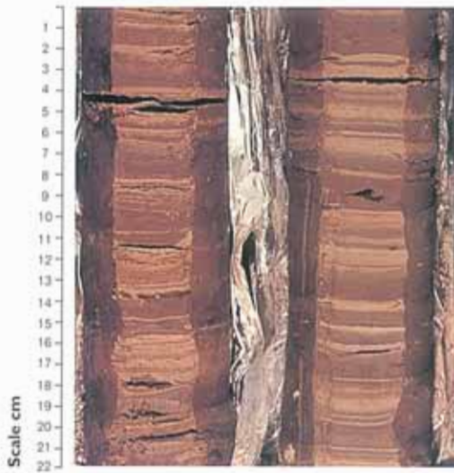
Borehole cores of glacial lake clays from near Killearn.
